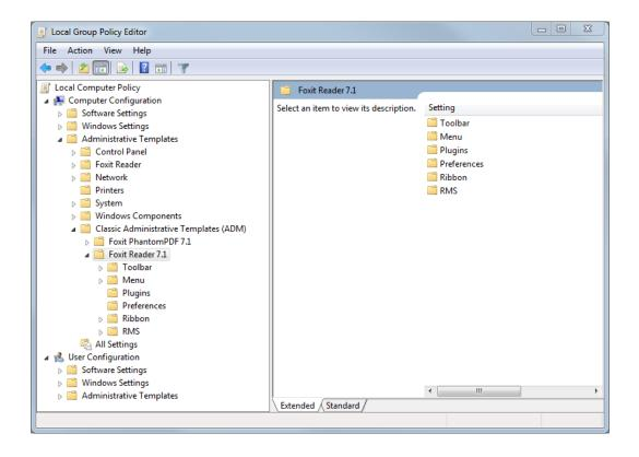
For .admx file, put the .admx file in C:\Windows\PolicyDefinitions and do the setting. The .admx file should be used in combination with an .adml file. And the .adml file should be put in C:\Windows\PolicyDefinitions\language. For example, if in the English OS, the .adml file should be put in C:\Windows\PolicyDefinitions\en\_us.
